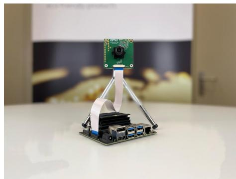
Figure 6: ams OSRAM image sensor connected to an evaluation kit.
